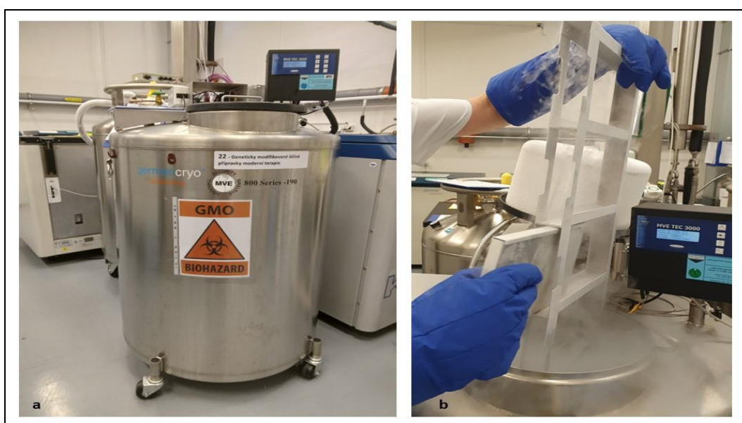
Figure 2 a. Liquid nitrogen container MVE (Chart, Bio Medical Ltd., USA) that uses „dry-storage“ technology; b. detailed close-up view on the frame in the interior of the container (Source: Tissue Establishment CZ000426, Czech Republic).
