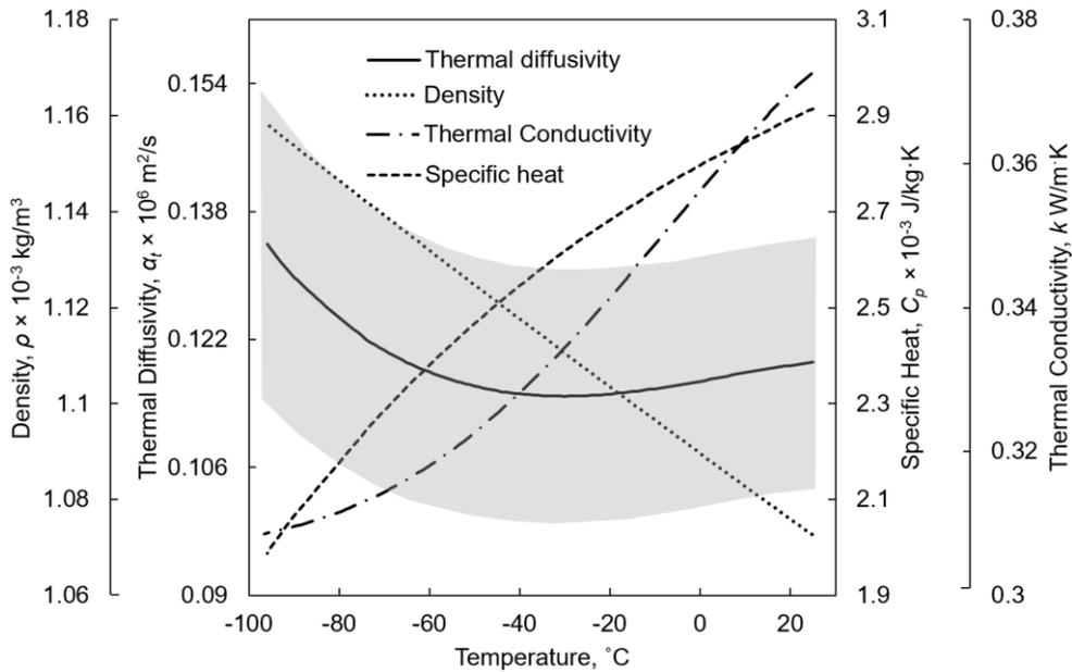
**Figure 4.** Thermophysical properties for 7.05 M DMSO, where the density and thermal diffusivity are compiled in the current study, while the thermal conductivity (7) and specific heat (42) are taken from literature data. The uncertainty in thermal diffusivity estimation is displayed by the gray region.
