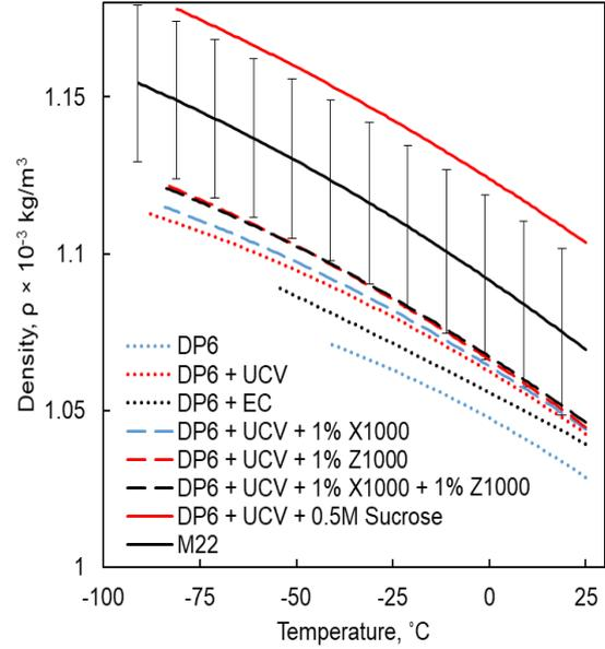
**Figure 1.** Density of CPA+SIM cocktails in higher cryogenic temperatures, where the coefficients for polynomial approximations are listed in Table 1.
